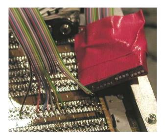
With this I characterized the core memory timing, I tried to identify important lines, refined my schematics and connected a logic analyzer to all vital signals. In applying different patterns, I already discovered read instructions, 2-cycle instructions, read-modify-write instructions and some instructions freezing the unit and requiring a power cycle (not only a reset pulse<sup>3</sup>):
