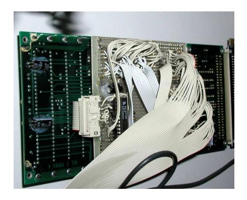
During this process I refined my schematics again, analyzed the ALU and the timing generation and made more professional connections to the logic analyzer:
